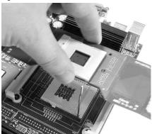
You may need to bend the flexible "wings" of the interposer upward.
