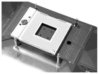
**7** Close the the socket on the target system.
