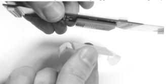
**4** Align the interposer over the socket on the target system.
