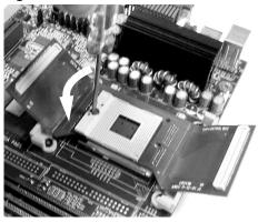
**8** Align the processor over the socket on the interposer. Gently wiggle the assembly until you feel the pins fall into the holes. Visually check that the bottom of the processor module is flush with the top of the socket on the interposer, then close the socket.
