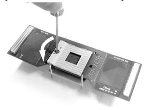
**9** Align the processor over the socket on the interposer. Gently wiggle the assembly until you feel the pins fall into the holes. Visually check that the bottom of the processor module is flush with the top of the socket on the interposer, then close the socket.
