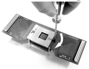
Insert a narrow, flat blade screw driver through the hole in the interposer.
