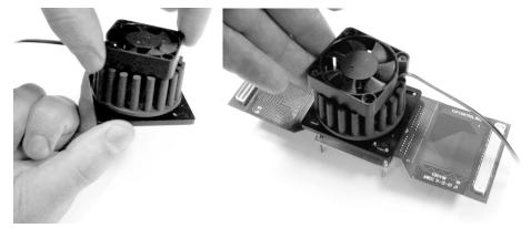
Tip: Rotate the top portion of the heatsink counterclockwise before installing it, then re-tighten the heatsink once it's on the interposer.
