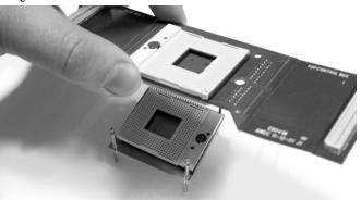
You may need to bend the flexible "wings" of the interposer upward.
