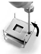
**5** Align the interposer over the socket on the target system.
